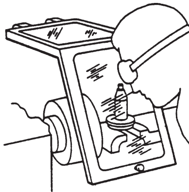
Figure 19. Plexiglass guard on lathe protects operator from flying chips
