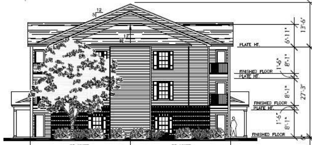
2 BUILDING #1&#2 – TYPICAL END ELEVATION
