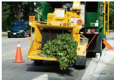
Self-feeding wood chippers commonly are used in tree trimming operations. With chipper discs or drums spinning at anywhere from 1,000 to 2,000 rotations per minute, the equipment can be very dangerous if not handled properly.
