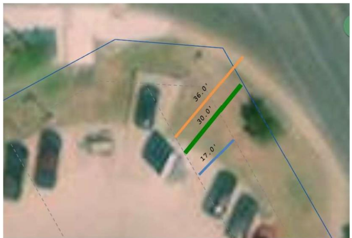
501 N Bryant Blvd CAR TOWN HYUNDAI Existing Pylon to be Refaced Overall Height = 30' Setback from curb = 36' Setback from Property Line = 30' Max Height Allowed = 50' Setback from Lot Line = 17'
